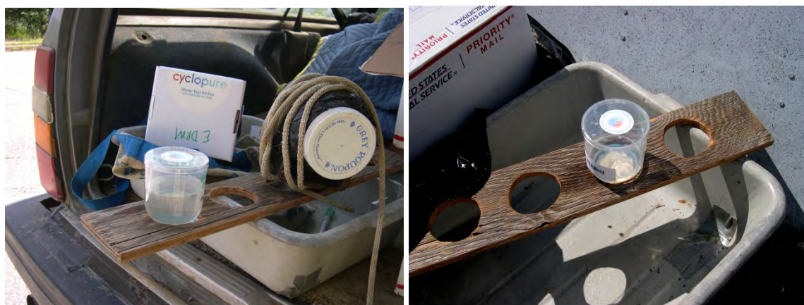
Figure 2: Cyclopure water test kit, drain board and throw bottle.
